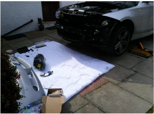
Now that both the headlights and bumper are removed we can go about installing the Angel Eyes but before we do you will need to swap any existing bulds from your old headlight to your new DEPO
