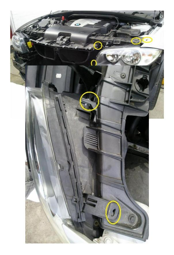
Having removed the 4 screws and loosened the 5th the headlight should then come away from the its mounting point. You may need to give it a firm pull to get it past the support bracket but dont be afraid to yank it hard if need be. (NB: The 5th screw may need to be loosened more to lower the support bracket. If you remove the 5th screw it is much easier to remove the headlight but accessing the screw with a
