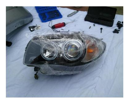
You will need to use the 25mm hole cutter to remove a part of the headlight backing plate so you can run the ballast cables through the
