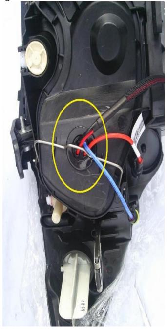
Make sure to flick the switch on the inside of the headlights to the up position for RHD vehicles
