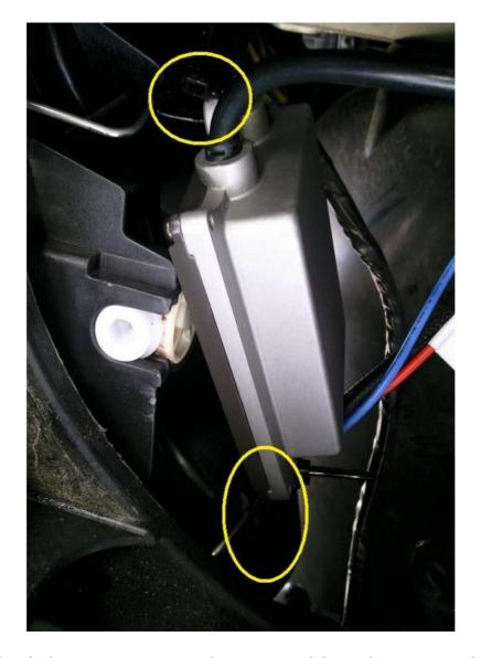
I then attached the wires as neatly as I could to the engine bay, again using cable ties. All wires and equipment are totally secure and there is no flapping.
