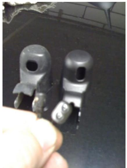
This picture, just shows the new nozzle in a little more clarity. The nozzle shafts are splined, so they just slide straight down. DO NOT TRY TO TWIST THEM when pulling the old one out or pushing the new one in, otherwise this could ruin them.
