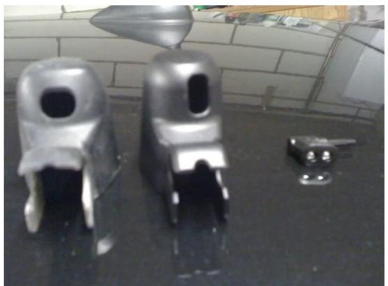
And here is the new nozzle in place, with its cover. The new nozzle just pushes down and the cover clips over as per the old one. Now it just takes a bit of time and patience to angle the nozzles so they squirt onto the window as you want them. I found a safety pin ideal to move the nozzle around in its housing.
