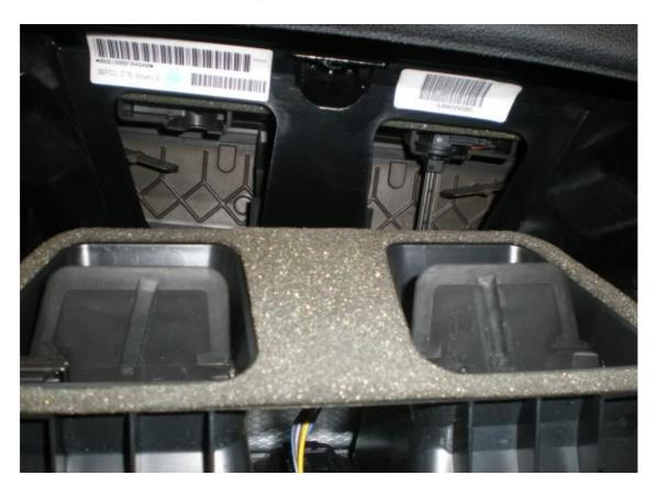
The easiest (imho) way to route the wire from here is (as you look at the dash) down to the left towards the glovebox. Here you can see a fuzzy black wire. This is the wire which controls the hazards, DTC and lock doors function. The satnav wire needs to follow this wire, but then drop straight down as if it were going down the right hand side of the glove box.
