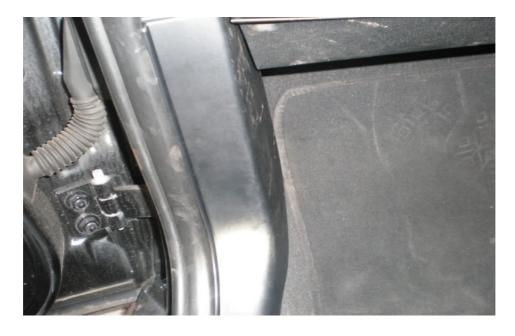
With the cover removed, it is easy to see where the wire can be routed.
