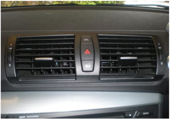
The airvent is a complete module, which has 4 retaining tabs at the top. Simply press down and pull out towards you, so the bottom of the module pivots.
