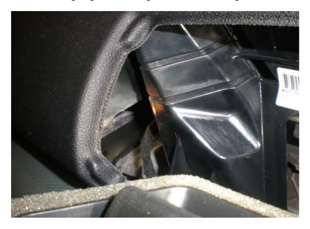
The next issue is how to get the wire into the glovebox as at first it appears to be a self contained unit. It is not! looking into the glove box, you can see an access panel at the rear left handside.
