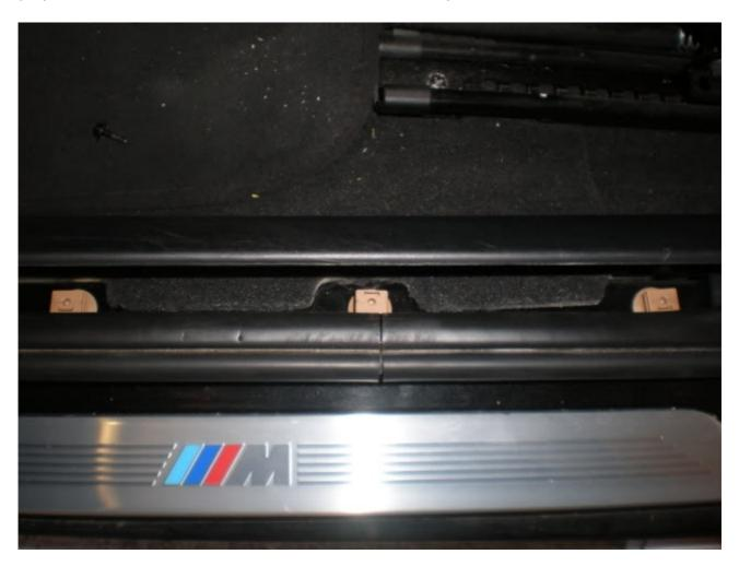
Once the sill cover is off, the a pillar cover will pop off too. This is held in place by two retaining clips, so the whole unit can be carefully pulled out.
