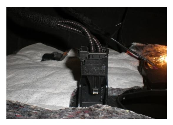
Now you will be able to thread the satnav wire down through the air vent and then route it through to the glove box. You will find that the wire is just long enough to reach the glovebox access panel. Here you will need a cig lighter extension cable and plug it in as below.
