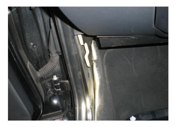
Then it is simply a case of running the (extension) wire under the carpet/sound proofing and then under the passenger seat, under the armrest and into the cig power input next to the aux input.
