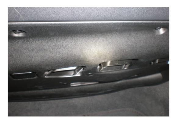
This panel clips onto the centre console by a plastic push through pin, which has a centre plastic capped rivet. This is a pain to remove, but i did it using a small flat bladed screwdriver to pull out the centre pin, which looks like this.
