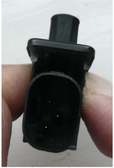
Pressing on just the easier rear clip with a finger could be enough.
