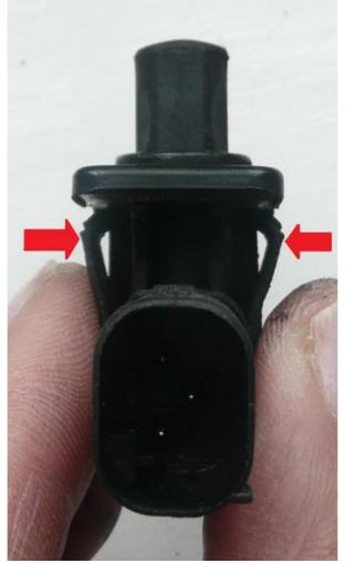
To remove the switch out of its seating, you are supposed to press on both holding clips to free the switch from the mounting.
