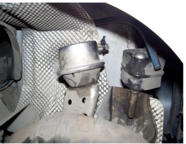
6. Now, plug the golf tee into the vacuum hose to prevent dirt and dust making its way up the vacuum hose:
