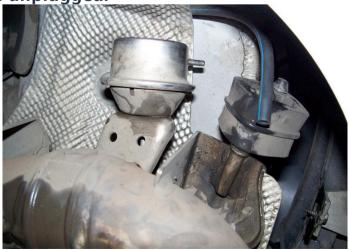
5. Now cut a piece of the clear plastic tube, about 4cm long. You are going to use this to plug over the actuator where the vacuum hose came off. This is to prevent dust and dirt making its way into the actuator. Push the piece of plastic tube over the actuator, then bend it in half, and secure it with a cable tie. See the picture below:
