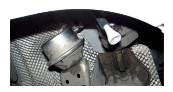
7. Lastly, what I found to work quite well is to tuck the vacuum hose + golf tee into the rubber mounting of the exhaust bracket. It fits in nicely and doesn't rattle around underneath the car:
