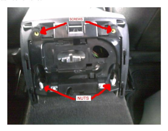
Fit armrest into the console then fit screws and nuts.
