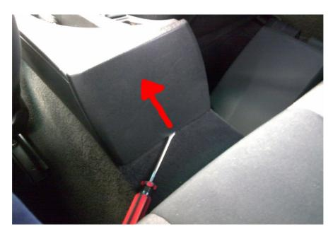
Then remove the two nuts and two bolts, and remove the plastic plate buy lifting the console up and pulling the plate down and manouver it so it can be removed.
