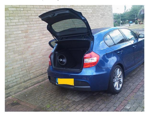
Its a sealed box and so doesnt have a port (air port to release the air from the rear of the sub when in action). A ported enclosure would have to be bigger in volume and I was already limited for space
