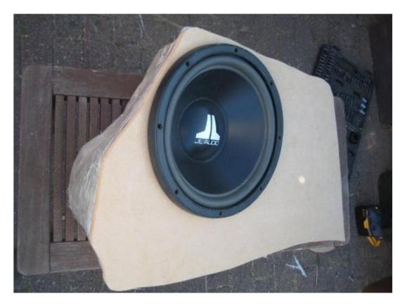
Now you have the front baffle squaring up with the shell its time to get the P38 out to fill the gap between them. Using masking tape secure the front baffle to the shell all the way round from the outside.(sorry no pictures of this stage).
