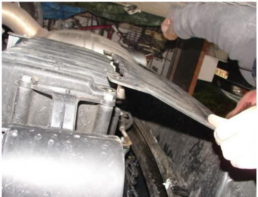
Once you have removed the screws, it is a case of gently easing the bumper off its mounts. The bumper clips in on the side of the arches and needs to be teased out slowly. You will see that the bumper tucks in under some trim in the middle part. This just needs to be lifted out and the bumper will slide out.
