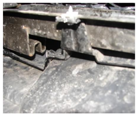
Once this trim is removed, you are left with removing the main bumper, there are a number of 8mm screws to undo. There are 3 screws under each main arch, and quite a few underneath the connecting trim. There are also 3 10mm screws there as well! The underneath of the car looks something like this... you should be able to see some of the screws...
