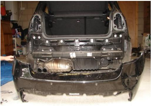
REMEMBER!!! not to pull away too quickly as you will need to unclip your rear number plate lights and reversing sensors. These are just very simple clips that you push in and pull out.
