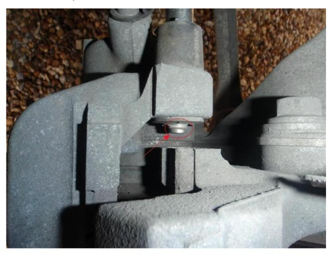
5. Now it is necessary to remove the retaining clip. This can sometimes be a bit tricky but after years of practice I fnd a correct size fat head and a pair of pliers do the job quite nicely as pictured below.
