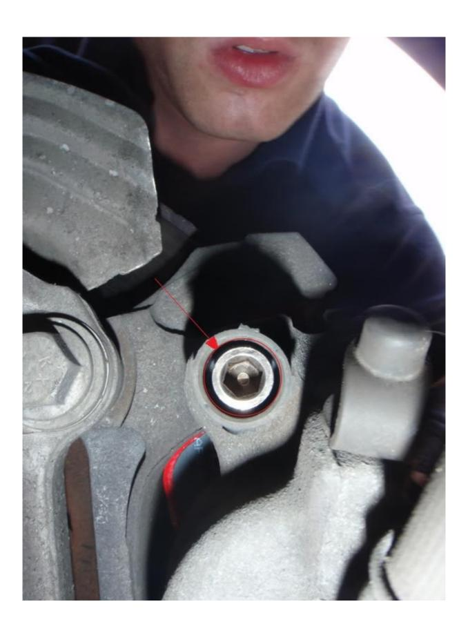
4. Fully undo both Allen bolts and push them all the way back (I carefully use a medium size fat head on the exposed thread) you need to do this so they won't interfere when trying to slide the calliper out of it's bracket.
