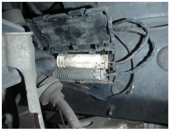
6b. The rear brake wear sensor simply unclips along it's entire length but... To access the termination box (located where the red dot is) requires a bit more work. It is necessary to partially unbolt the wheel arch lining (six 8mm self tapping bolts) which isn't difcult, just more of a nuisance! Pictured below
