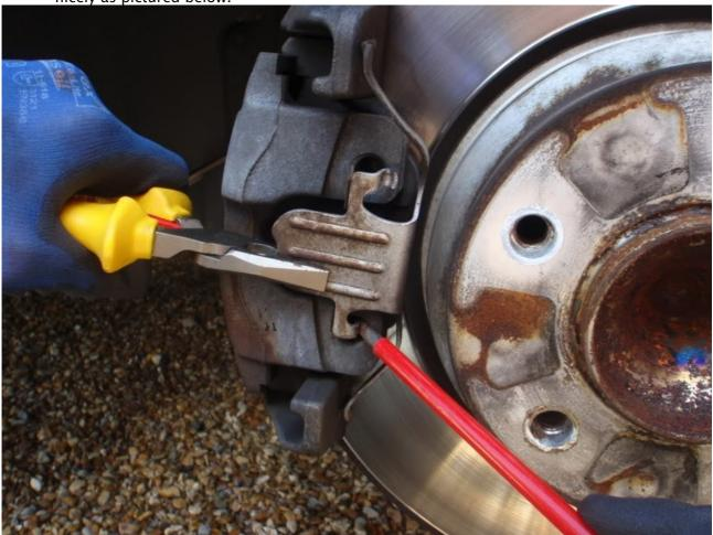
6a. If the calliper you are working on dose not have the brake sensor go to step 8. The brake wear sensor on the front is on the passenger side. On the rear it is on the drivers side. Only one per axel (2 in total). This is a lead that simply unclips along it's entire route to it's termination box. The front is very easy to access and just unclips.
