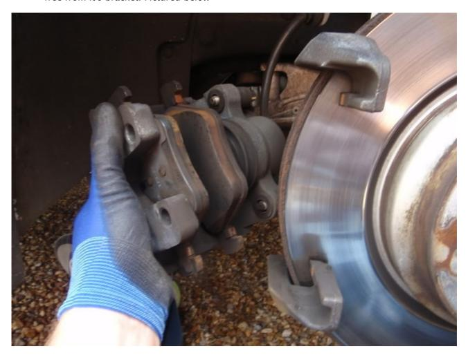
9. The pads should now be free to pop out of the calliper. Once both pads are removed the brake piston will need to be pushed all the way back in to accommodate the new unworn pads. I use a simple but efective piston compression tool available from good car maintenance stores however. A large set of pipe grips or even a 'G clamp' can be used (I don't recommend the later thou)
