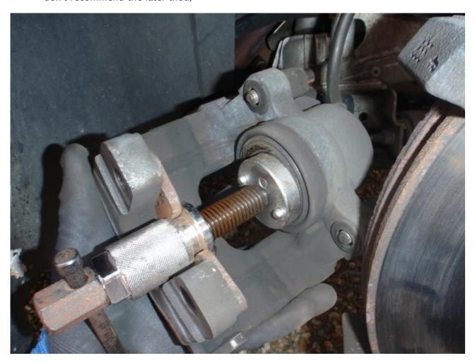
10. Once compressed the new pads should be installed with the clip removed from the old pad and installed on the new (note: copper slip is often used on the back of the pads to eliminate squeaks)
