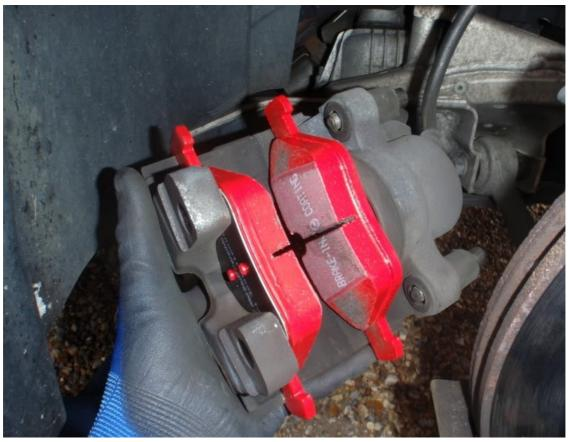
11. Now it is a simple case of reversing the process remembering to re clip the new brake sensor onto the pad.
