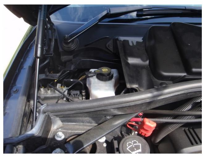
2. Remove the brake fuid reservoir cap and place a rag in/around it to save it spilling over your engine bay when you compress the calliper pistons!
