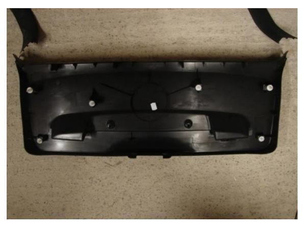
At this point I didn't remove the trim, I went on to undo the side pieces of trim, which again have poppers, but are only held on by 1 screw each, which doubles as the holder for the boot cover.
