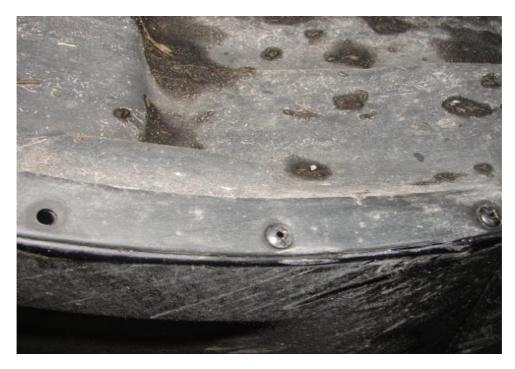
Just place a skewer into the centre and the little plastic rods pop out and can be recovered once you've taken the inner arch off.
