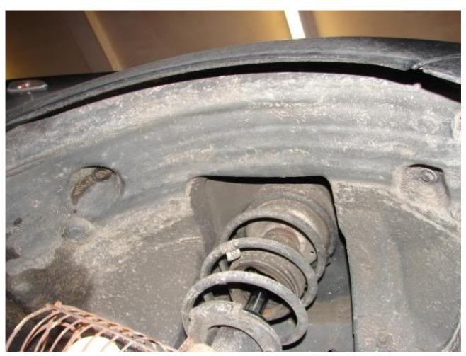
There are quite a few screws and bolts to undo here, but you only need to remove the inner arch behind the wheel.
