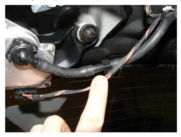
By doing this on a number of occasions and blowing through to into the wiper, i cleared any blockage and it now works perfectly!
