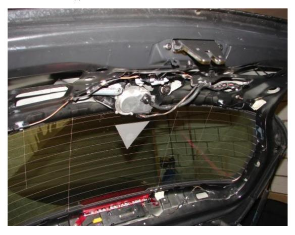
I decided to undo the non-return valve (as pointed out) and see if water would come through, which it did, although very soapy. (bear in mind i only refilled with clean water)
