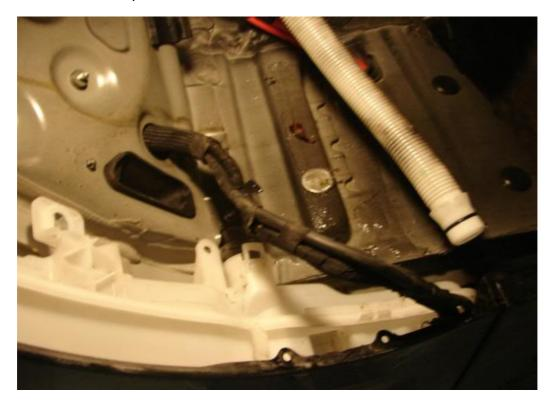
Now you can slide out the water bottle. It is connected by the two water pipes to the washer jets, a low level water sensor and the indicator loom. There is no way you can get confused with the electrics as the male and female connectors are colour coded! Thanks BMW! You'll see i've put a bit of masking tape on the water pipe that goes to the black pump. This was to make sure i didn't accidentally cross them over when putting them back together.
