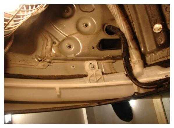
also at this point, you need to disconnect the concertinaed white filler tube. This simply unclips and needs a bit of force to push out.
