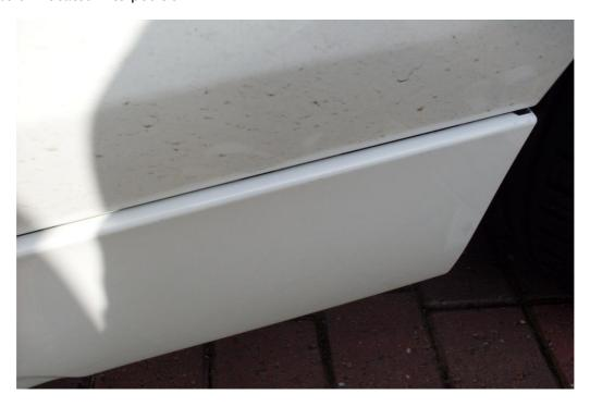
Pic shows only 1 clip secured to sill, push gently to fully locate sill to body
