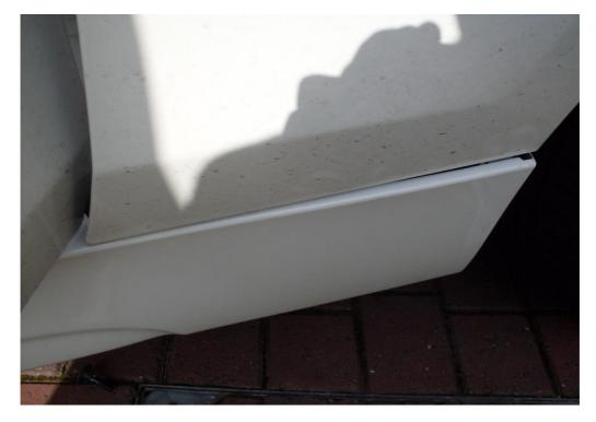
**Step 9**Fit the datum scrivet (4th fixing car rearward) followed by the remaining 4 scrivets in any order.
