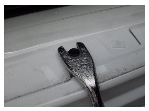
**Step 3**Remove the 5 scrivets from the body with the trim fork.
