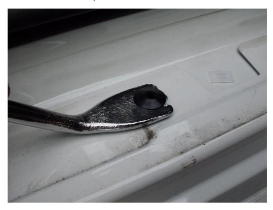
**Step 4**Underneath the car you will see 10 TX25 fixings, these need to be undone using a ratchet and the TX25 bit. Once removed gently remove the lower edge of the sill from between the body and the under-body protection panel, this will make it easier to remove after the next step.
