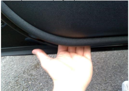
6. The door card should hopefully then come off! I didn't bother un-clipping any wires and just got someone to hold the card whilst I added the new tweeter. You can see where the tweeter plugs into, indicated by the red circle.
