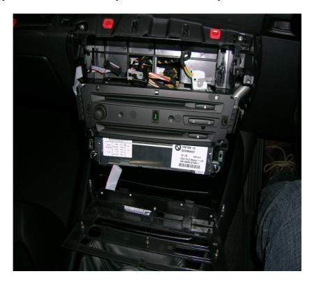
6. With the radio removed you simply use a radio mute lead (no cutting of wires required) and refit in reverse. The only think you will have to do is provide a switchable live from the cigar socket. The easiest way to achieve this is to unclip the Idrive button and the steering gaiter, in front. Connect to the thick Green wire you find below and fish the wire back through to the rear of the radio.
