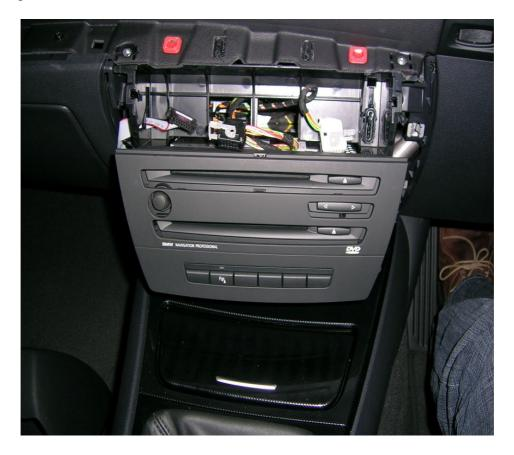
5. Now remove the 4 screws securing the DVD CD unit theses are located adjacent to the chrome portion of the unit where you can see the BMW parts labels
