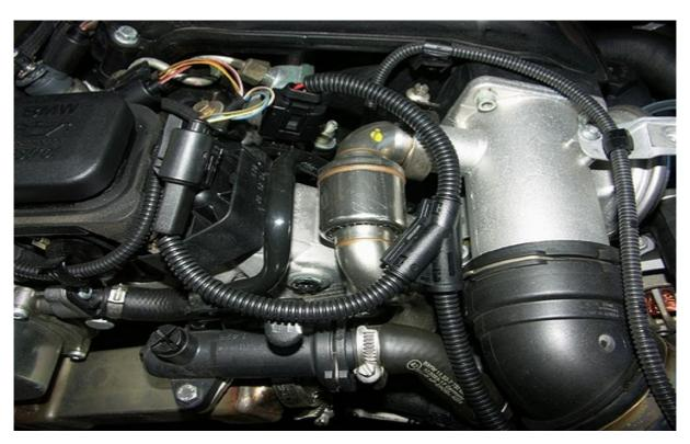
Where to put the actual tuning box? This is where the optional waterproof protector sleeve comes in handy. It has a zip-tie at the neck which I have attached to the right hand side of the engine here:
