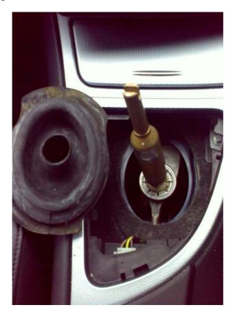
3. Undo the white collar around the gear lever 'ball' and lift the lever up to gain access to the clip on the change rod underneath
