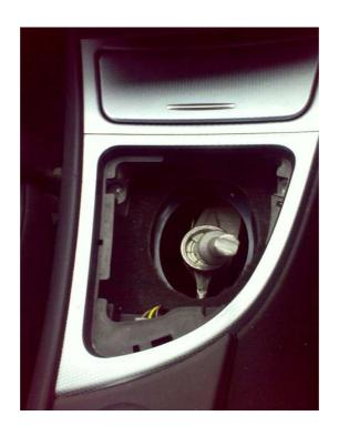
9. Refit the rubber surround onto the base of the lever
