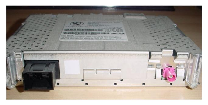
The tuner bolts to the bracket with 3 bolts that use an 8mm socket:
