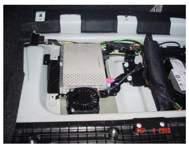
I then luckily found out how to remove the side cover next to the rear seat. It was actually too easy. I removed a few panels before realizing you just pretty much pull from the top. It pops right out. This is the first view of my MOST bus:
