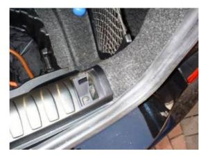
Remove 2 trim plugs (a trim plug removal tool is useful for this to avoid damage to the trim) from the tailgate scuff plate and remove trim.
