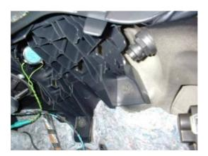
The shelf can now be removed from the car to remove the standard shelf and speaker. Be careful though, if the loadspace lamp has been on the whole time it will be damn hot as I found out On the right hand side shelf the PDC speaker (business HU only) will need to be removed. Then fit upgrade speaker/tweeter and work in reverse to re-assemble.
