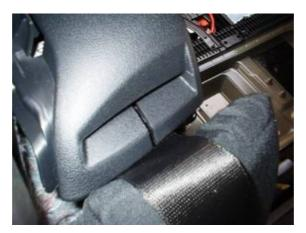
Slide rear trim out of location on underside of shelf trim by sliding the lower part of the rear 1/4 trim inboard
