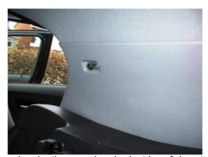
Remove the door aperture seal and tailgate seal on both sides of the trim, there is no need to remove all of it. Gently remove the trim from the sides so as not to touch the headlining and lever the trim inboard from the top.
