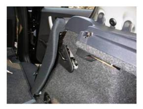
Remove striker loop Torx fixing and loop trim.
