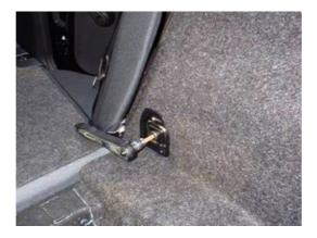
Gently lift off the 2 covers on the tailgate scuff plate with a flat blade screwdriver and be careful not to slip. Remove 2 screws.
